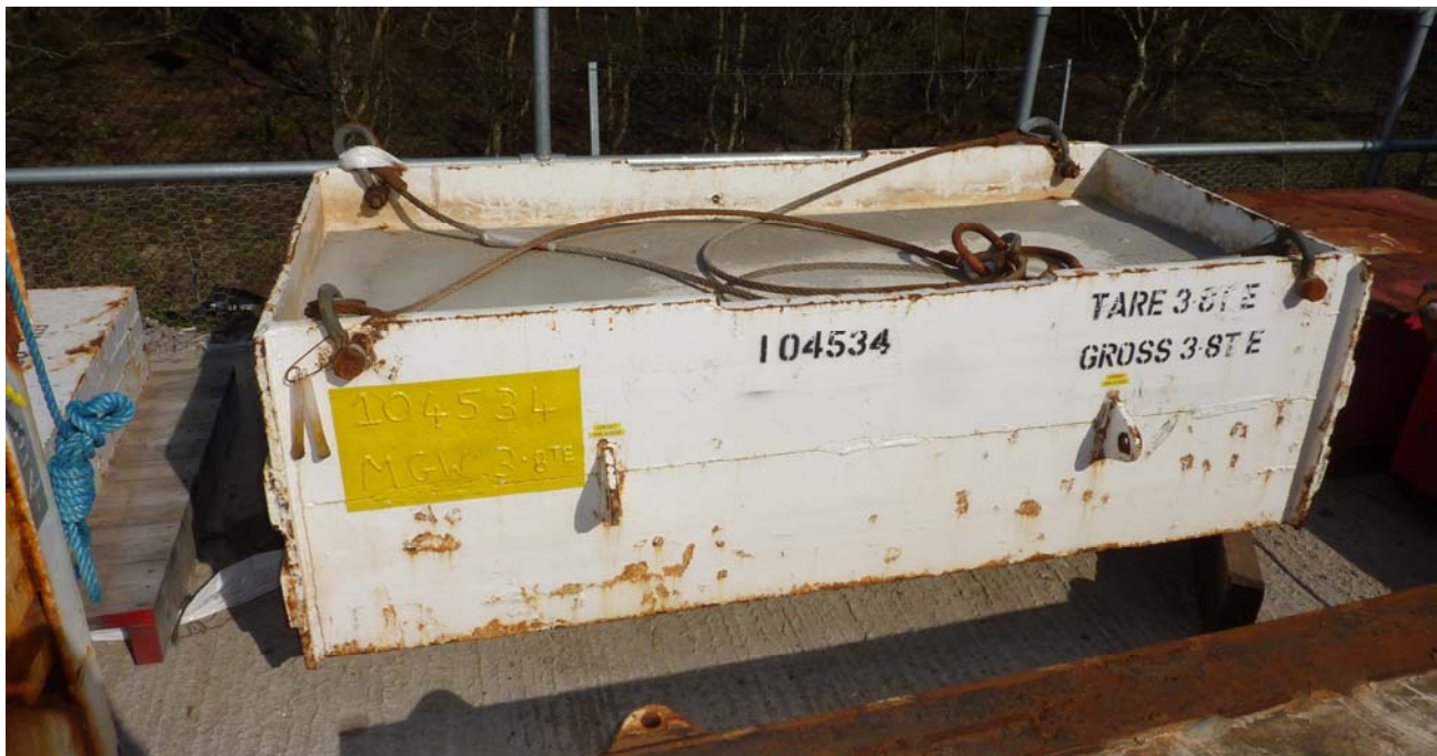
Figure 5.1 Photo of 3.8-tonne Clump Weight
