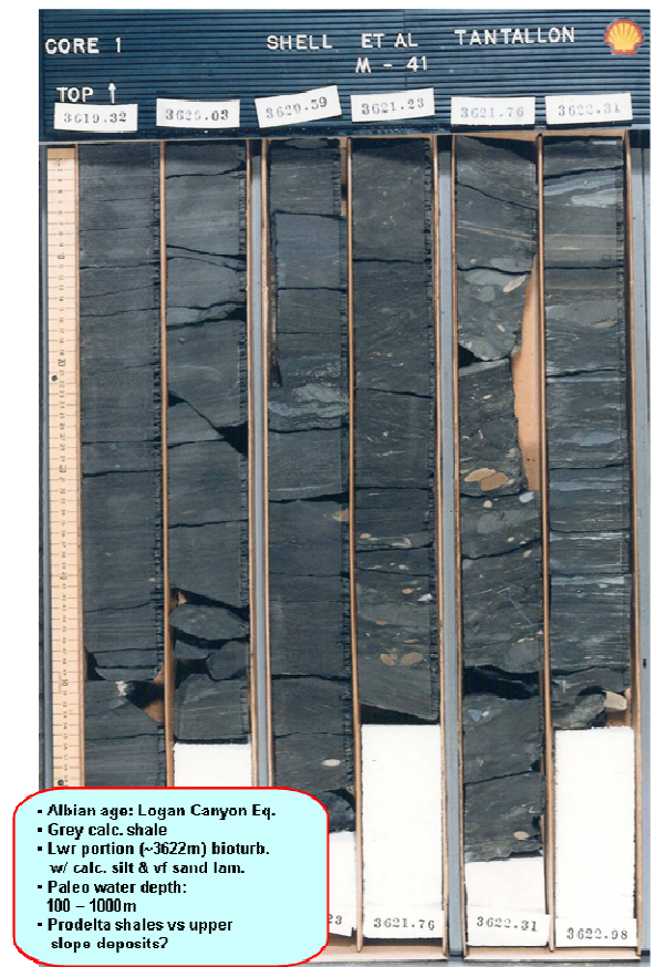
Figure 80. Tantalón M-41: Portion of Core #1 (3600.0 – 3627.0 m, 23.5 m recovered).
