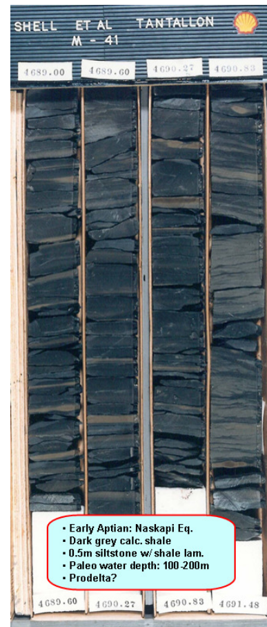
Figure 81. Tantalón M-41: Portion of Core #2 (4689.0 – 4717.0 m, 28.0 m recovered).
