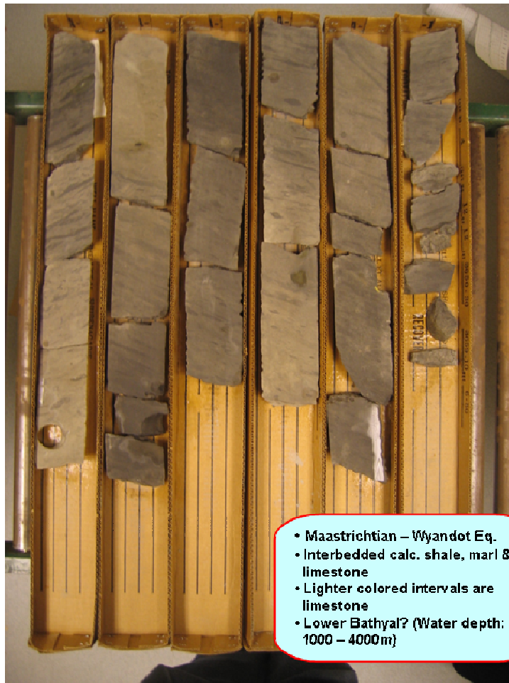
Figure 53. Shubenacadie H-100: Portion of Core #4 (3650.3 – 3659.1 m, 6.8 m recovered).
